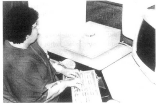
Fig. 3 Typist addressing the keyboard with the Penny and Giles "M" Series twin axis goniometer attached to her wrists
